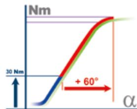
Tightening with torque and
