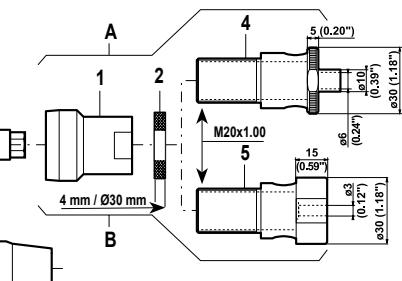
615 396 069 0: Machined routing kit for burr, max ø 6.4mm (1/4")
