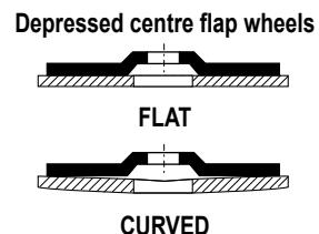
**Caution:** comply with the speeds recommended by component and abrasive manufacturers.
