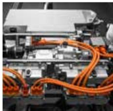
During the **assembly of components exposed to high voltage such as busbars and harnesses**, using insulated tools is one of the many important steps to protect from electrical shocks and damages:
